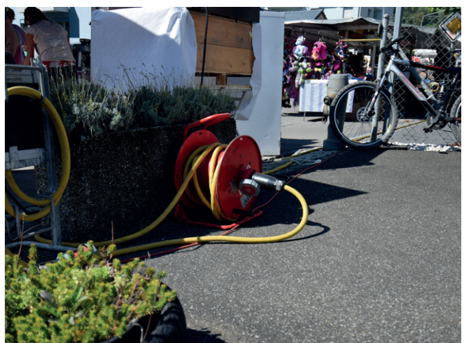
Cable reel with a metal body
